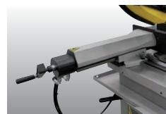
Mechanical stops for a fast head rotation at 0°, 45°, 60° and -45° degrees.
